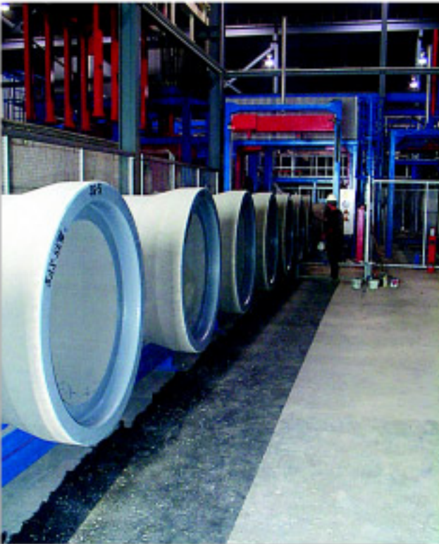
Royal's new Sblusselbauer Exact 2500 production plant produced the 36-inch diameter RCP used for the Wilmes Lake Sanitary Sewer Trunk deep installation project.
